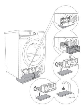
Open the outside cover. Hold the levers on the inside cover and rotate them as indicated by the arrows.
